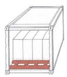
Securing of cargo towards the door: The free space between the cargo and the corner posts is filled in using squared lumber.
